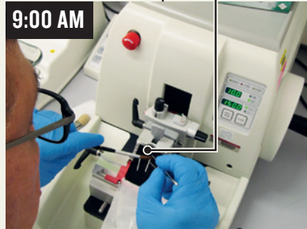
The clock starts ticking in earnest when scientists shave off slices of the paraffin block that contains the tumour to begin extracting DNA and RNA. Exposure to air can alter molecules and even change genetic sequences.
